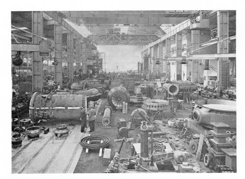
Fig. 9. From the fitting shop. The spiralcasing of a Nea turbine in the background left and the runner in the center of the picture.
